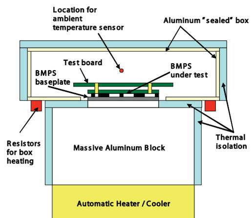
Figure 2 - Cross-section of the test equipment
