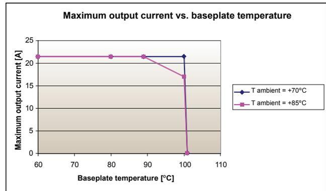
Figure 3 - PKY2616PI Available output current vs. baseplate temperature at  $V_{in}=27\text{ V}$
