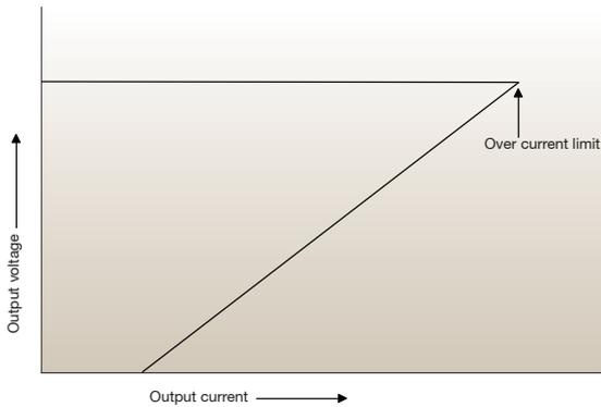
Figure 10 - Example of Over Current Protection with fold back limiting
