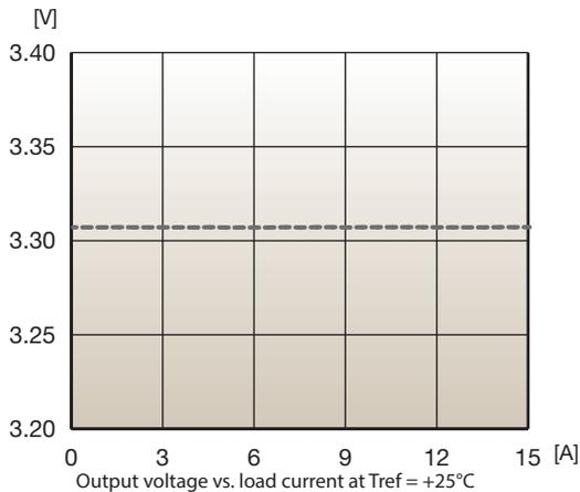
Figure 6 - Example of load regulation for DC/DC power module with synchronous rectification
