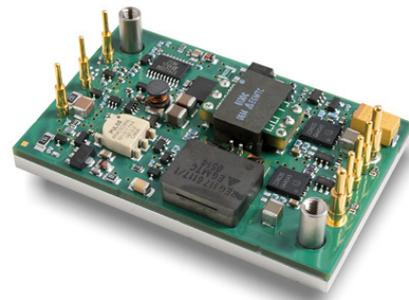
Figure 1 - Example of DC/DC converter
