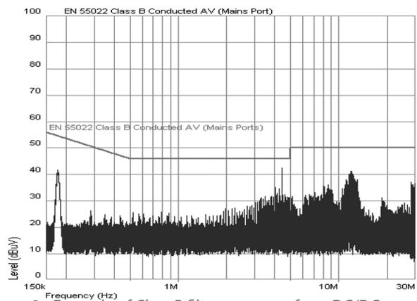
Figure 3 - Example of Class B filter response, from DC/DC converter technical specification
