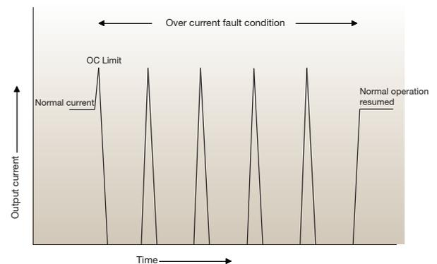
Figure 9 - Example of Over Current Protection with hiccup limiting
