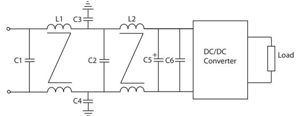
Figure 2 - Example of EMC filter design, from DC/DC converter technical specification
