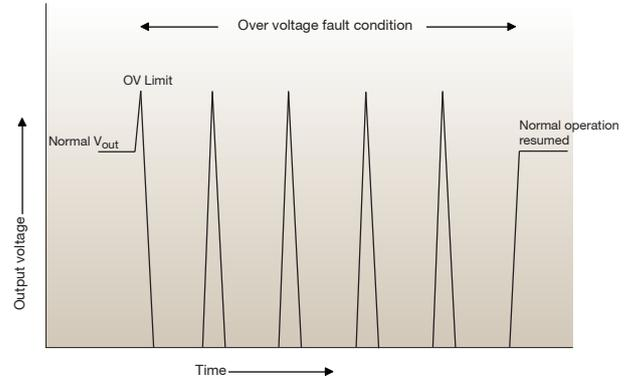
Figure 8 - Example of Over Voltage Protection with automatic recovery
