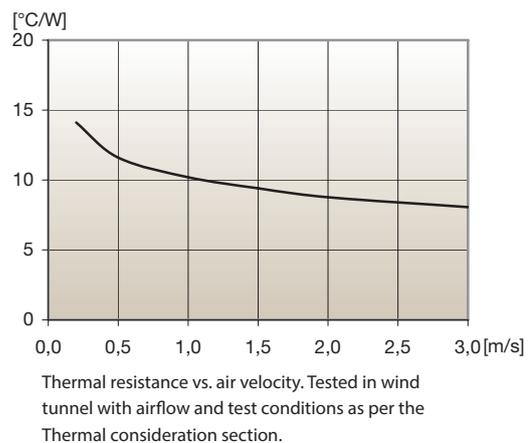
Figure 7 - Example of thermal resistance curve
