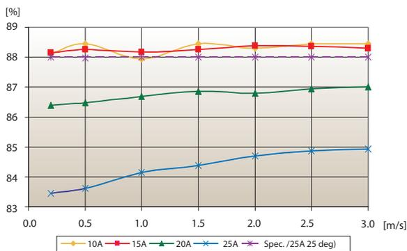
Figure 5 - Efficiency vs. Airflow Example.
