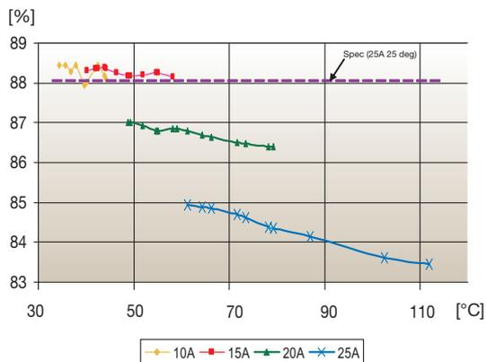
Figure 6 - Efficiency vs. PWB Temperature Example.
