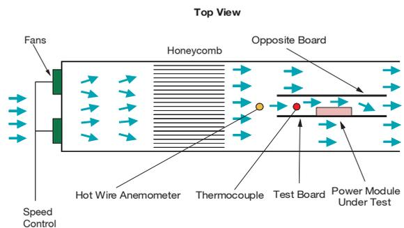
Figure 2 - Wind Tunnel Configuration.
