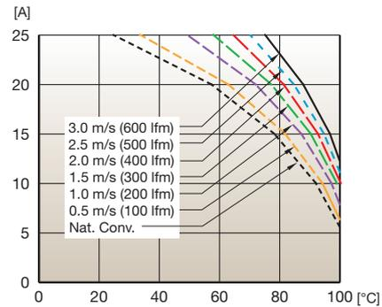
Available load current vs. ambient air temperature and airflow at  $V_o = 53$  V. DC/DC converter mounted vertically with airflow blowing from output pins to input pins.
