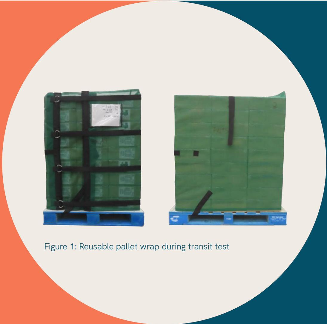
Figure 1: Reusable pallet wrap during transit test
