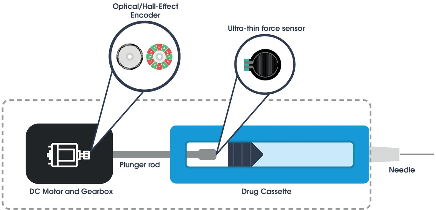
Figure 3: Autoinjector system design with rotary encoder and force sensor.
