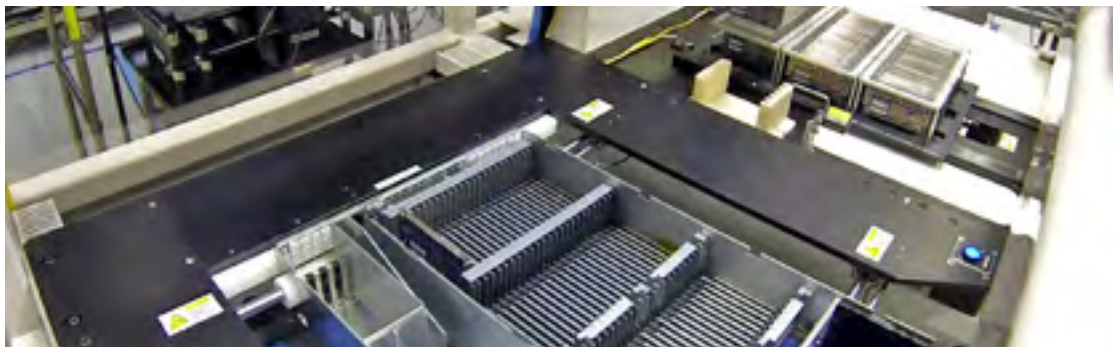
Robot inserts DIMM into Backplane Chassis
