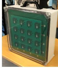
Customizable reference design for a Massive MIMO antenna array with 16 dual polarized elements, operating at 2.5 GHz
